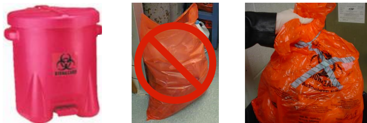
Figure 12.2 – (Left) Labeled red container with lid for accumulating biohazardous waste (other than regulated sharps). (Center) Biohazard bag outside of a hard-walled container, which is unacceptable. (Right) Infectious waste bag that was sealed, marked with heat-sensitive tape, and autoclaved.
