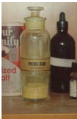
Figure 11.3 – A bottle of dried-out picric acid, which has become a highly shock sensitive Division 1.1 explosive (Photo courtesy of Robert Burke, www.firehouse.com )
