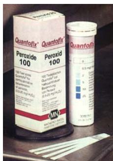
Figure 13.2 – Quantofix® peroxide test sticks. These strips are colorimetric, and can detect peroxides at a range of 1- 100 mg/L.
