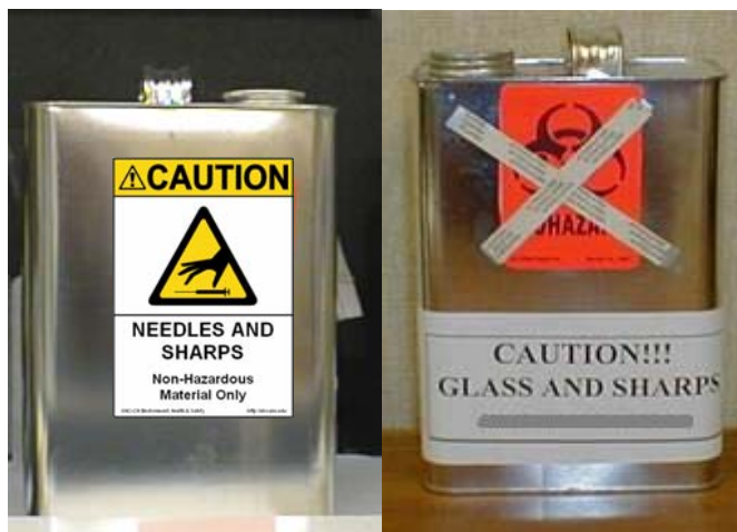
Figure 12.7 – Metal containers for disposal of regulated sharps. (Left) Metal can labeled for disposal of non-infectious regulated sharps. (Right) Metal can labeled for disposal of infectious sharps that has been autoclaved; autoclave tape over the biohazard symbol indicates contents are no longer infectious.
