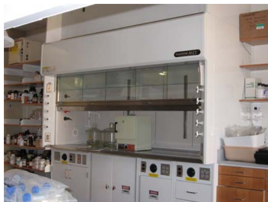
Figure 17.3 – Combination sash hoods. (Left): Correct position of a combination sash while performing experiments. (Right): Only raise the vertical sash when setting up experiments.
