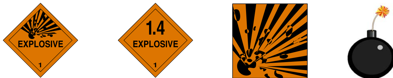
Figure 11.1 – Common placards and pictograms for explosive materials (left to right): DOT placard for Division 1.1 – 1.3 materials; DOT placard for Division 1.4 materials; European Union glyph for explosive materials; iconic glyph for explosive materials.
