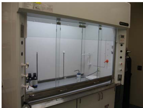
Figure 17.3 – Combination sash hoods. (Left): Correct position of a combination sash while performing experiments. (Right): Only raise the vertical sash when setting up experiments.
